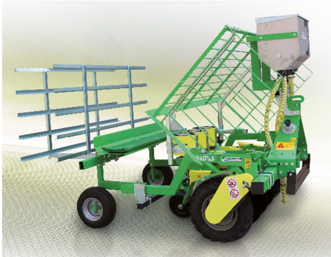
The transplanting machine PRACTICA MIDI, thanks to the round shape transplanting element with 8 cups with an interval moving, has a minimum row distance of 28 cm. It is optimal for small conical soil blocks. The share is equipped with a self cleaning system. The parallelogram system allows a uniform transplanting even on soils with irregular soil surfaces. Practica- Midi is equipped with a single plant tray holder and press wheels.
