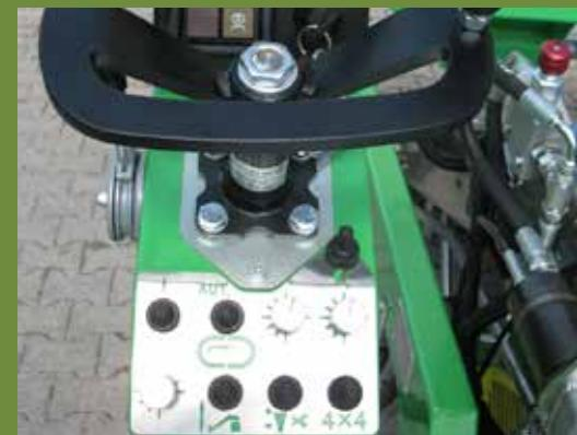
SISTEMA CON SENSORI ELETRO-IDRAULICI PER CONTROLLO ALTEZZA TAGLIO • ELECTRO-HYDRAULIC SENSORS DEVICE FOR THE CUTTING HEIGHT CONTROL • SISTEMA CON SENsoRES ELECTRO-HIDRAULICOS • CAPTEUR ELECTRO-HYDRAULIQUE PROPORTIONNEL • PROPORTIONAL-LEM ELEKTRO-HYDRAULISCHEM SENSOR • ЭЛЕКТРОГИДРАВЛИЧЕСКИЕ СЕНСОРЫ ДЛЯ КОНТРОЛЯ ВЫСОТЫ СРЕЗА
